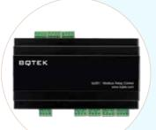
The BQ351-24 is a Modbus Slave IO module for interfacing to any PLC or PC using the Modbus RTU protocol. It behaves as a Modbus Slave Relay and Inputs. Outputs are controlled by writing to and reading from the Coils and Holding Registers. It can be used for many applications such as controlling lights and sprinkler systems, reading sensors and monitoring switches and other digital signals, or industrial control.
