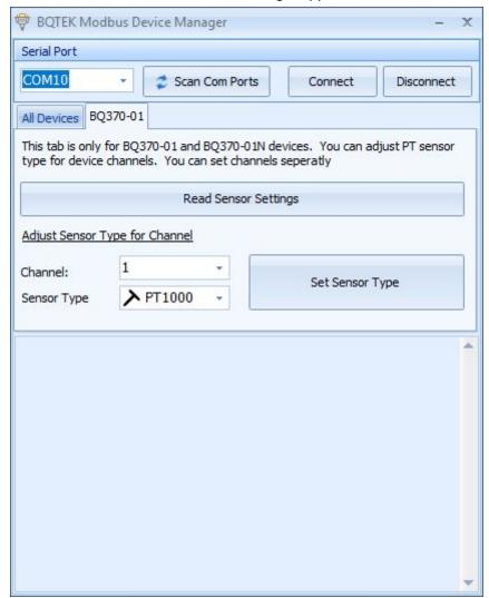
Put device to Settings mode as described before in this document. There is a tab in this software for BQ370-01. From this tab you can click "Read Sensor Setting" button for getting current sensor selections.
